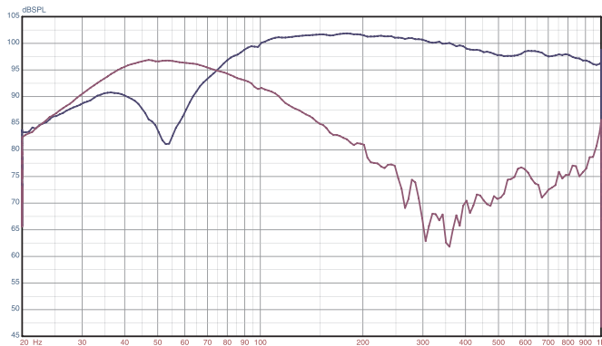
Figure 3. Nearfield frequency response of upper bass driver and upper reflex port. (Note data for port has not been re-scaled to compensate for differences in radiating area.)
